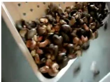
1) Feeding in machine the mixed kernels and shells.
