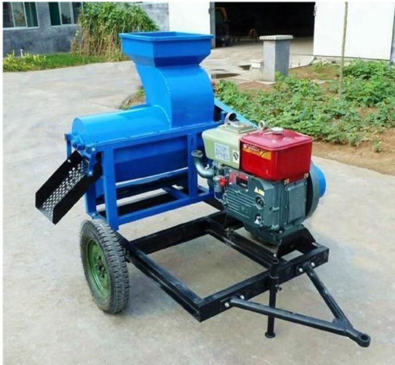
**Diesel type Corn thresher (backside view):**
