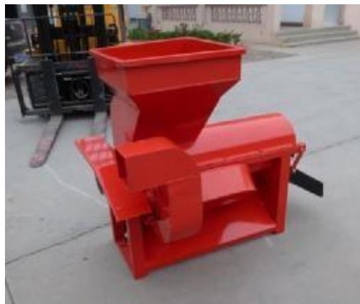
**The Thresher part (without engine/motor, without framework, without tire)**
